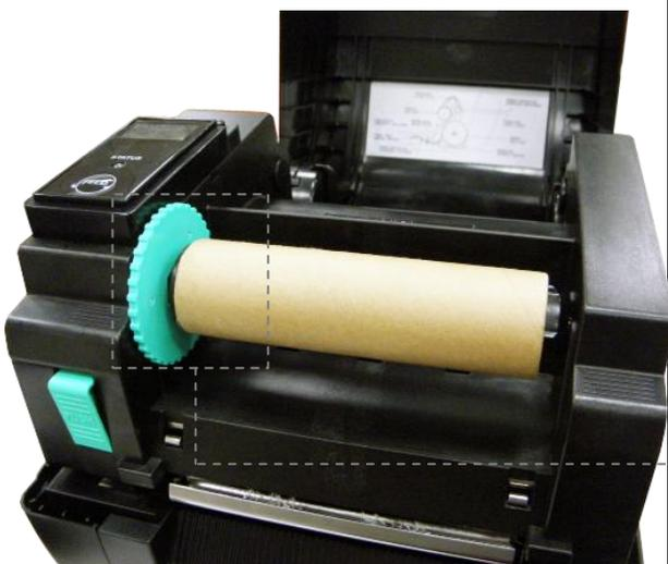
3. Insert the left side of ribbon rewind spindle to the ribbon rewind hub first then insert the right side of ribbon rewind spindle to the hole at the right side of ribbon mechanism.
