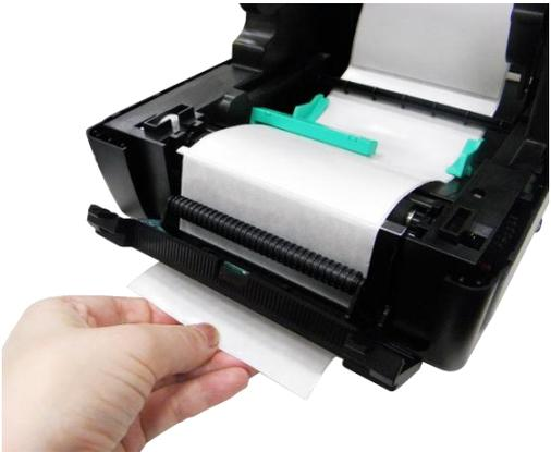
A side view of the printer with its lid open. The white liner is now loaded into the printer, and a hand is holding the end of the liner. |
