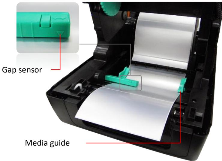
5. Feed the paper, printing side face up, through the media bar, media sensor and place the label leading edge onto the platen roller. Move the media guides to fit the label width.
