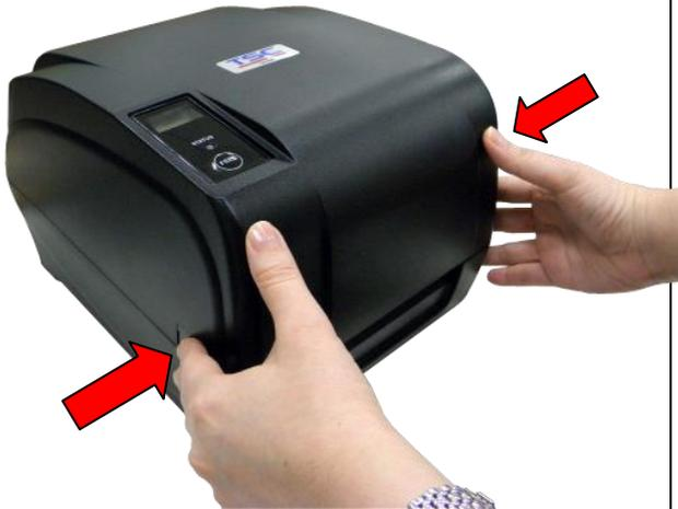
1. Open the printer top cover by pressing the top cover open tabs located on each side of the printer.
