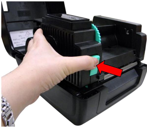
4. Push the print head release button to open the print head mechanism.
