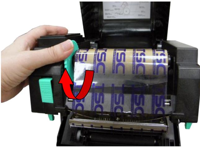
8. Turn the ribbon rewind hub until the ribbon plastic leader is thoroughly wound and the black section of the ribbon covers the print head.
