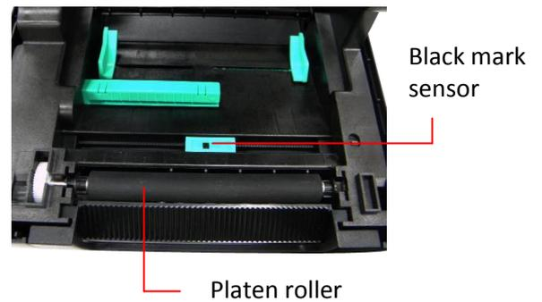
**Note: The media sensor position is moveable. Please make sure the gap or black mark is at the location where media gap/black mark will pass through for sensing.**
