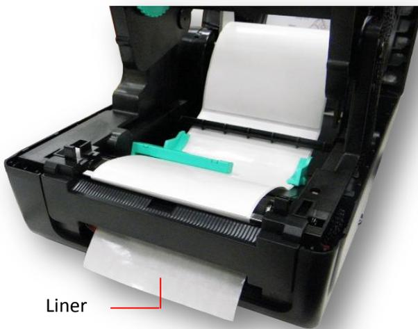
4. Close the peel-off module. Use the DiagTool to set the peel-off mode by selecting "PEEL" option for Post-Print Action setting then click "Set" button to enable the peel-off mode.
