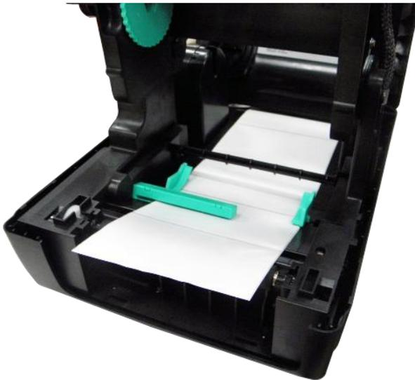
5. Refer to chapter 3.3.1 to install the label. Use “Diagnostic Tool” to set the media sensor type and calibrate the selected sensor.
