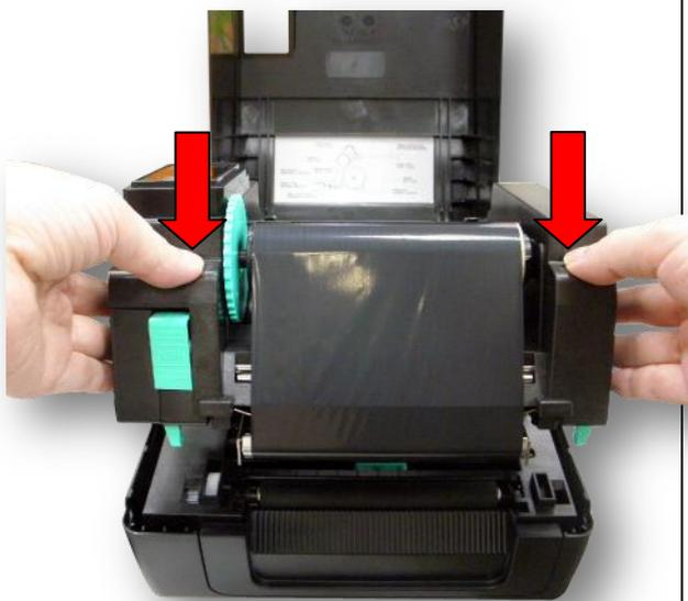
9. Close the print head mechanism by both hands and make sure the latches are engaged securely.
