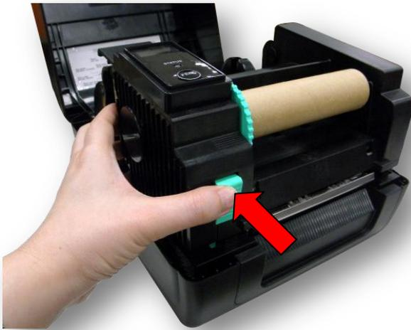
4. Push the print head release button to open the print head mechanism.
